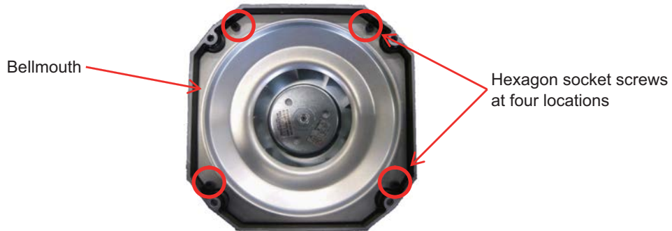
Cooling fan unit (before the bellmouth is removed)
